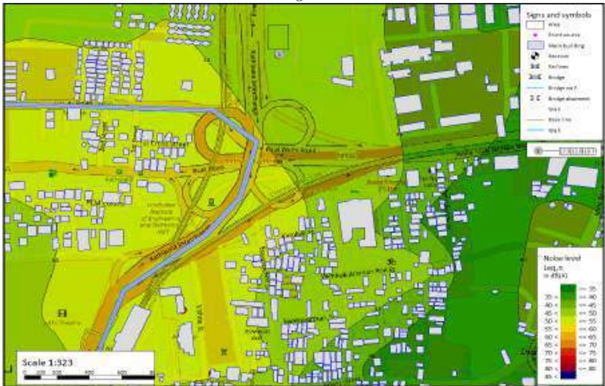
Figure 7-33: National School - Night time- Noise contour map for Operation phase after Mitigation
