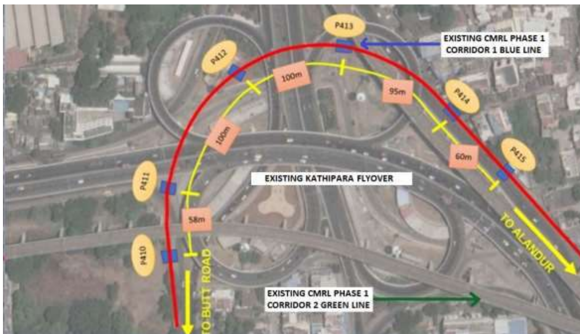
Fig. 3.9: Concept diagram of intersections between Proposed Kathipara GS and existing infrastructures
