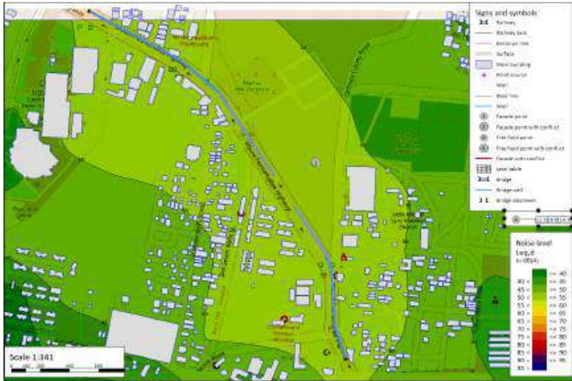
Figure 7-12: Contonement Board High School - Day time - Noise contour map for Operation phase after Mitigation
