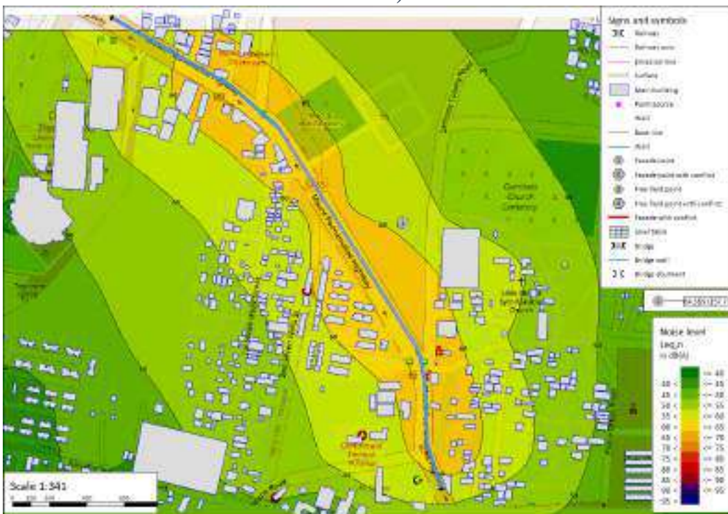
Figure 7-11: Night time Noise contour map for Operation phase (CTC to St. Wesley Church).
