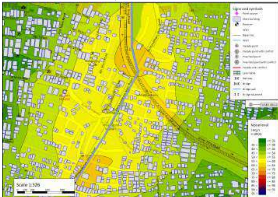
Figure 7-23: Night time Noise contour map for Operation phase (Adambakkam MRTS to Medavakkam Main road).
