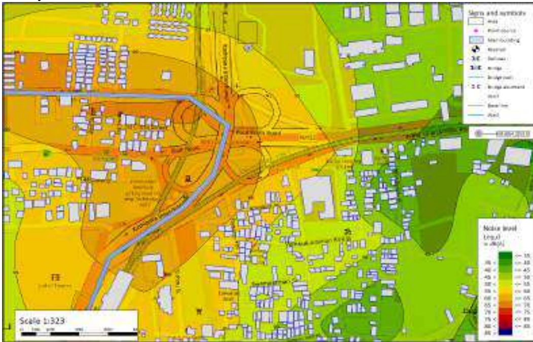
Figure 7-30: Day time Noise contour map for Operation phase (St. Wesley church to Alandur).
