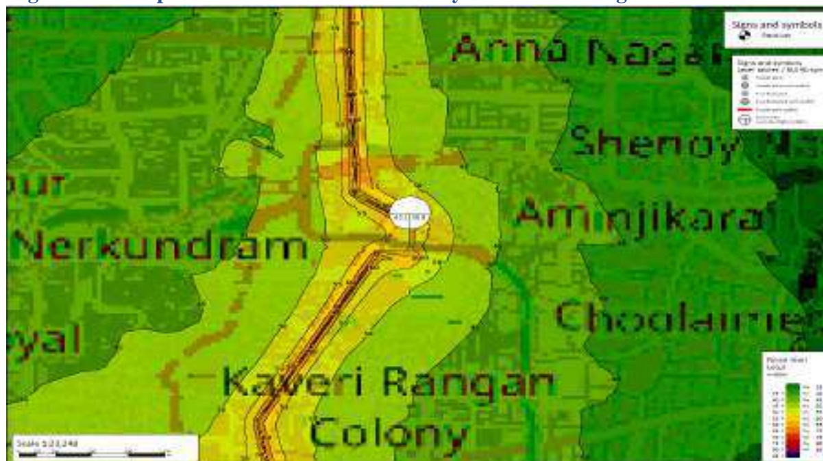
Figure 7-62: Operation Noise at HR-10– Day Time- No Mitigation
