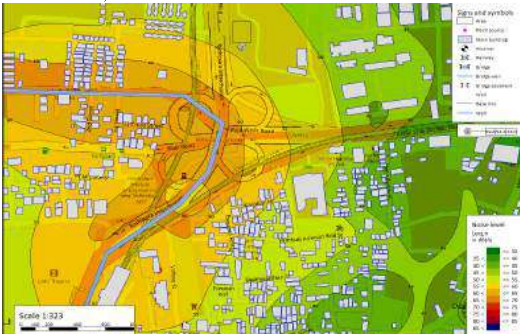
Figure 7-31: Night time Noise contour map for Operation phase (St. Wesley church to Alandur).
