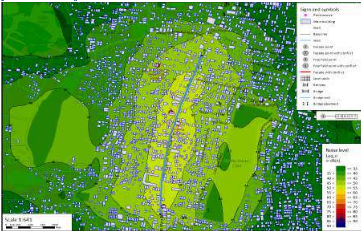
Figure 7-9: Anjakha Hospital Night time - Noise contour map for Operation phase after Mitigation
