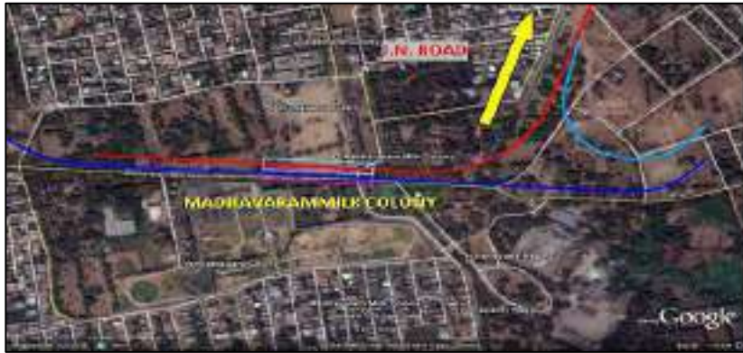
Figure 2-3: Switch Over Ramp from Elevated to Underground- ALIGNMENT CROSSING RAILWAY TRACKS AT VILIVAKKAM METRO
