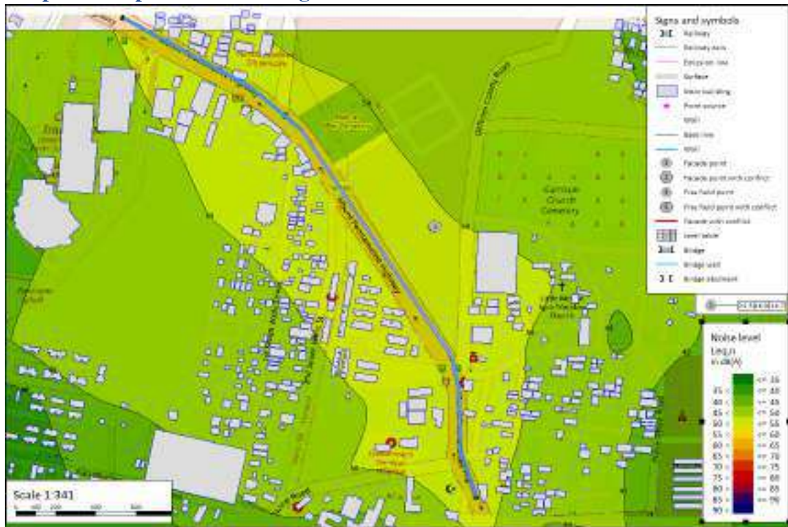
Figure 7-13: Contonement Board High School - Night time- Noise contour map for Operation phase after Mitigation
