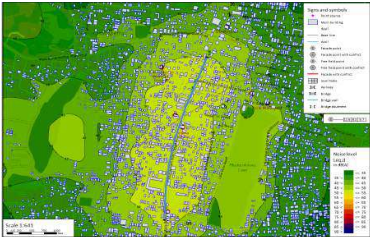
Figure 7-8: Anjakha Hospital Day time - Noise contour map for Operation phase after Mitigation
