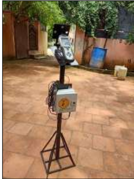
Figure 4-1 Photograph of instrument used for baseline Noise monitoring
