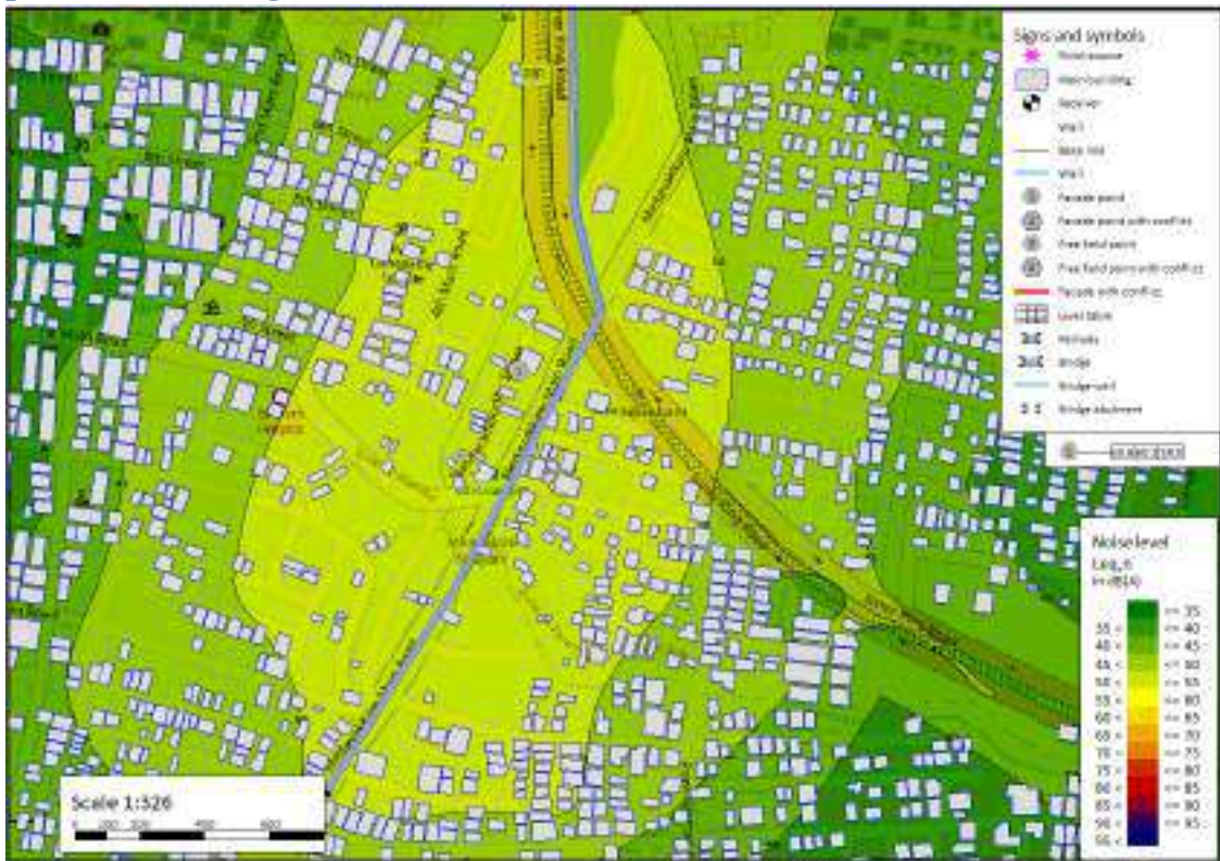
Figure 7-25: Kalpana Hospital - Night time- Noise contour map for Operation phase after Mitigation
