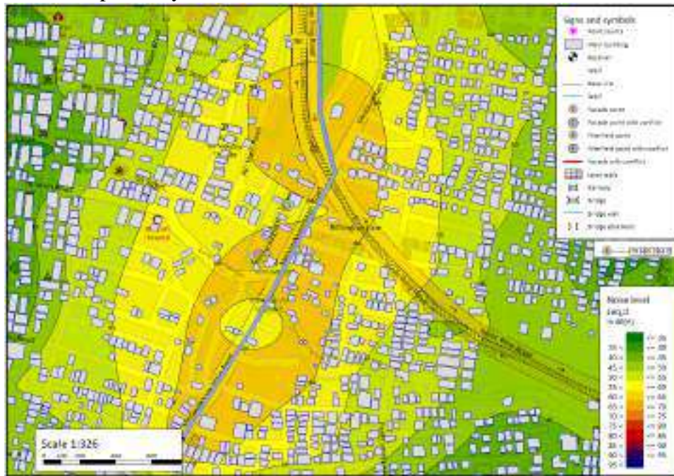
Figure 7-22: Day time Noise contour map for Operation phase (Adambakkam MRTS to Medavakkam Main road).
