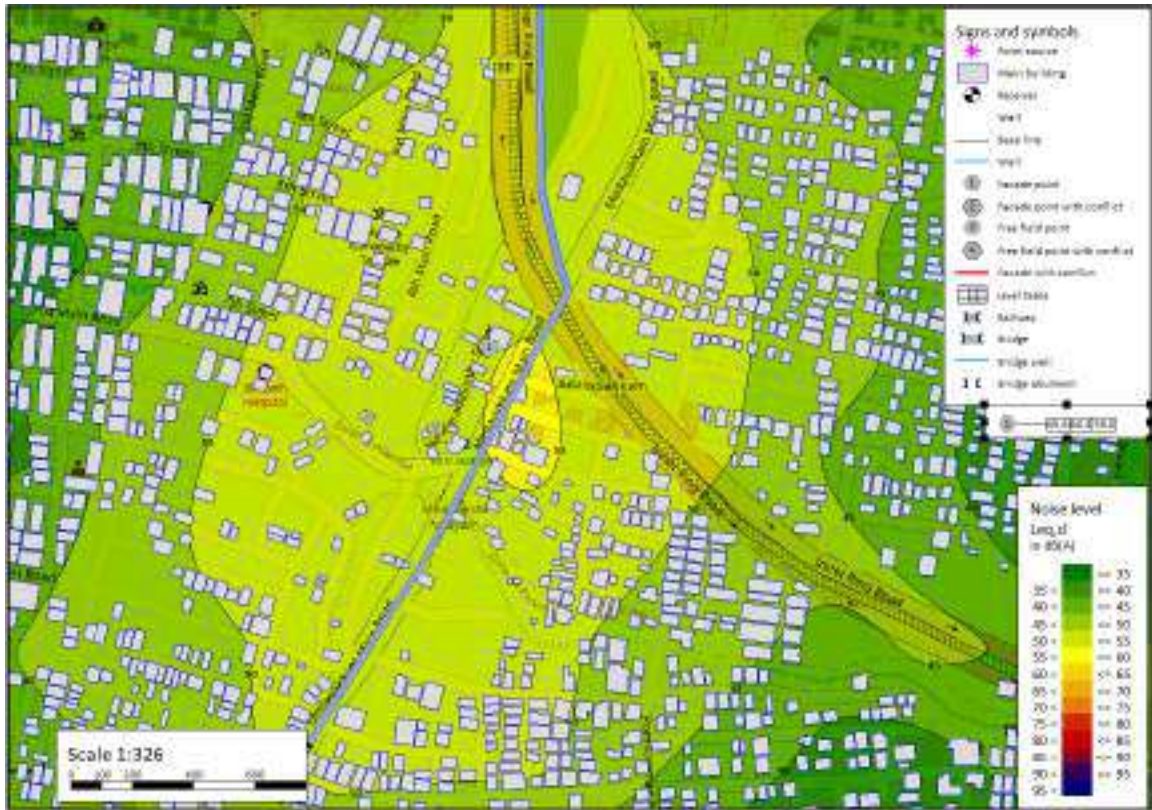
Figure 7-24: Kalpana Hospital- Day time - Noise contour map for Operation phase after Mitigation
