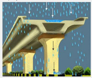
Concept Diagram - Rain Water Harvesting in Metro Via-
