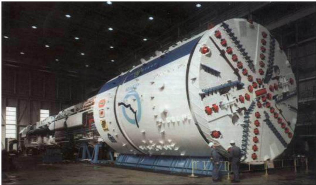
FIGURE 5.46: EARTH PRESSURE BALANCE TBM
