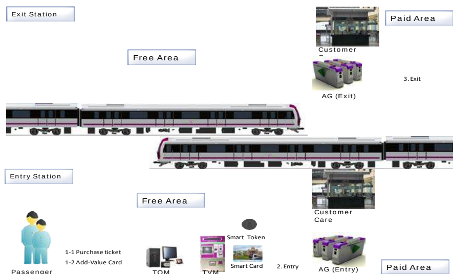
FIGURE 10.3: AFC SYSTEM ARCHITECTURE
