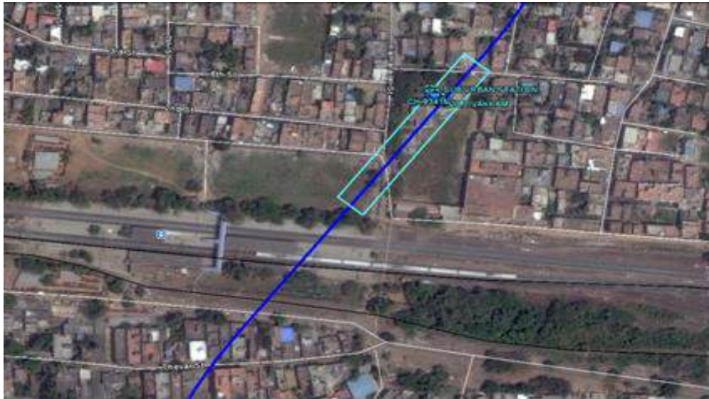
FIGURE 5.27: ALIGNMENT CROSSING RAILWAY TRACKS AT VILIVAKKAM METRO
